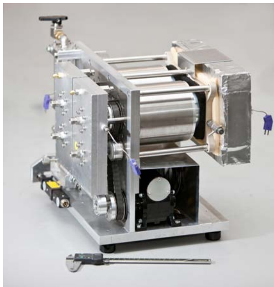
Figure 1. Two permanent magnet refrigeration systems (PM I and PM II) developed at UVic.
